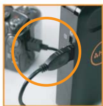
Set up the linking between digital camera* and WFT510
