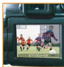
The DSC will switch to PictBridge Mode**. Choose the image and transmit to WFT510.
